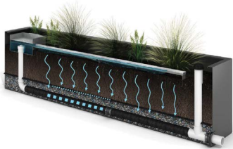
Water percolates through media and fabric.
