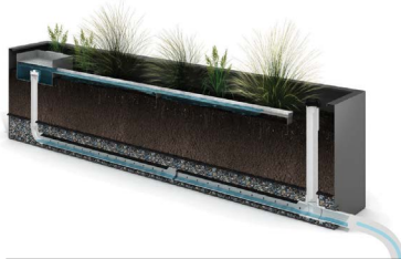
Water enters perforated drainpipe and exits.
