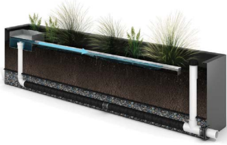
Water flows down the Level Spreader.
