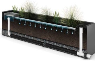
Water trickles through perforations into media.
